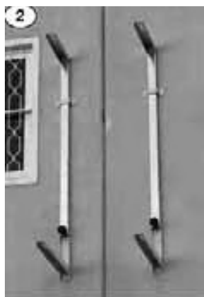
Step 2: Set the inverted squares on the wall supports and turn the handles to adjust them on the upper part.
